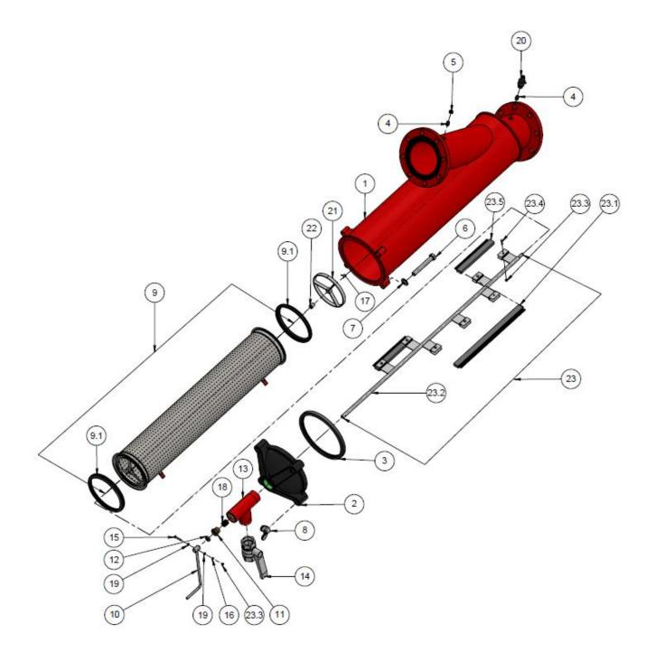
for amiad metal semi-automatic brushaway & scanaway filters steel & spare parts
