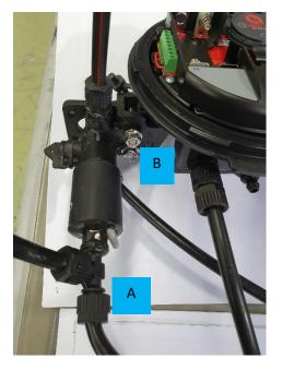
4. Assemble the new solenoid on the existing bracket and reconnect the red & black solenoid wires to the ADI-P inputs. Reconnect the control tube connectors (use Teflon on the threads)
