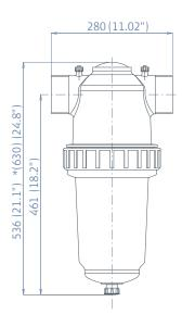
**Dim. In mm (inch)** \*Approx. length required for maintenance
