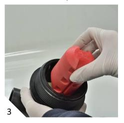
• Insert the Float halfway into the Body [1], insert the Clamping Stem into the Rolling Seal groove of the Body; make sure that it is inserted in the direction of the arrow [2]. Push the Float and the Clamping Stem together downwards into the Body until they are locked [3].
