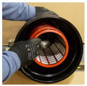
2. Reassemble the dirt collector and the centralized seat.
