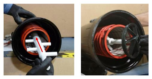
3. Assemble the cover to the filter body.
