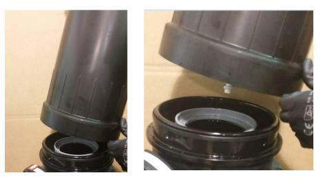
5. Hold the cover with two hands, turn it over the body in order to secure the bayonet connector [A], make sure the cover is correctly locked on the body [B].
