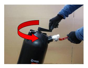
6. Close the flushing ball valve gradually.
