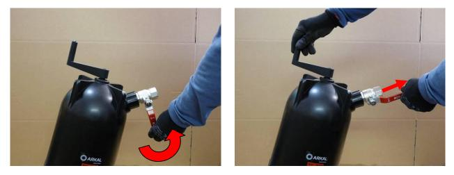
Water starts to flow out to the drain.
