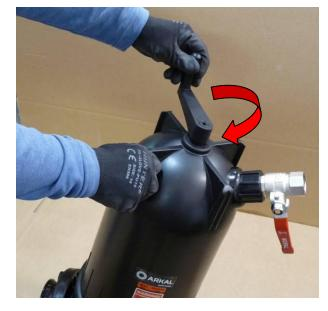
7. Return the dirt collector inward to the rear side of the filter by turning the handle clockwise until it stops (don't use force).
